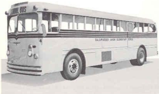
HALL SCOTT UNDERFLOOR POWER 232 AND 240 H.P. 61 to 79 PASSENGER CAPACITIES DOUBLE DOOR REAR LUGGAGE COMPARTMENT OPTIONAL
