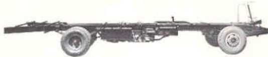
INTEGRAL CHASSIS AND BODY CONSTRUCTION— SIDE MOUNT RADIATOR LOWEST FRAME HEIGHT—THREE STEP ENTRANCE
